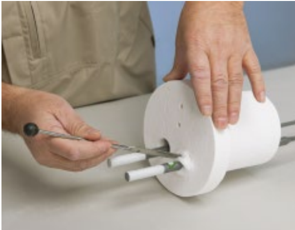
4. After packing heavy-duty ceramic fiber loosely into the recesses of the terminal holes...
