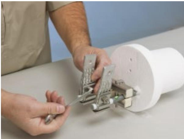
6. When determining the position of the element holder, it is of the utmost importance to ensure that the tapered transition between terminal and heating zone comes fully below the hot face of the furnace lining. If not, there is a risk that the part of the heating zone which is inside the lining may become overheated. When connecting the installed elements, the aluminum braids should first be bolted to the elements and then to the busbars.
