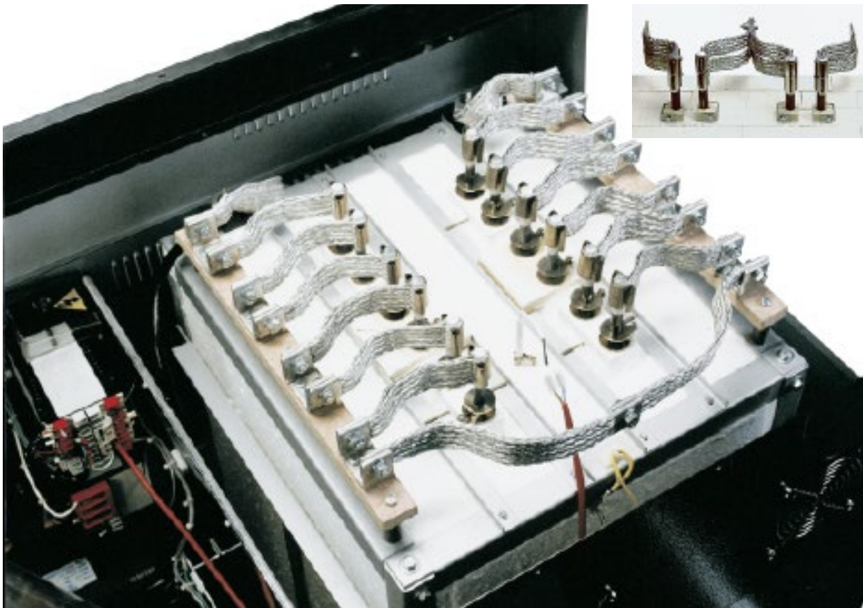
Kanthal® Super elements connected to busbars.
